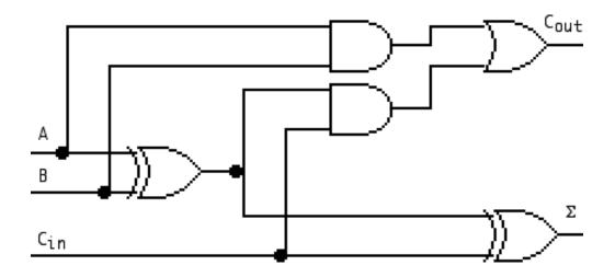
Suppose that the propagation delays for the and and or gates are 0.1 ns each, while that for the xors is 0.2 ns. (XOR requires a more complex circuit). Then the delay from A or B to Cout is max(0.1 + 0.1 ns, 0.2 + 0.1 + 0.1 ns) = max(0.2, 0.4 ns) = 0.4 ns.
